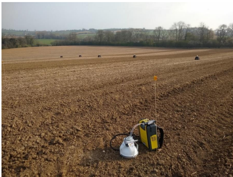
Figure 2: 9-metre wide plough and direct drill plots running across the field, with Gasmeter gas analyser sitting on a ring measuring field greenhouse gas flux.
